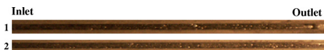
Fig. 10. Photos taken at 1800 s: (1) I=600 \text{ mA cm}^{-2} and u_{\text{O}_2} = 2 \text{ m s}^{-1} and (2) I=1200 \text{ mA cm}^{-2} and u_{\text{O}_2} = 5 \text{ m s}^{-1} .
